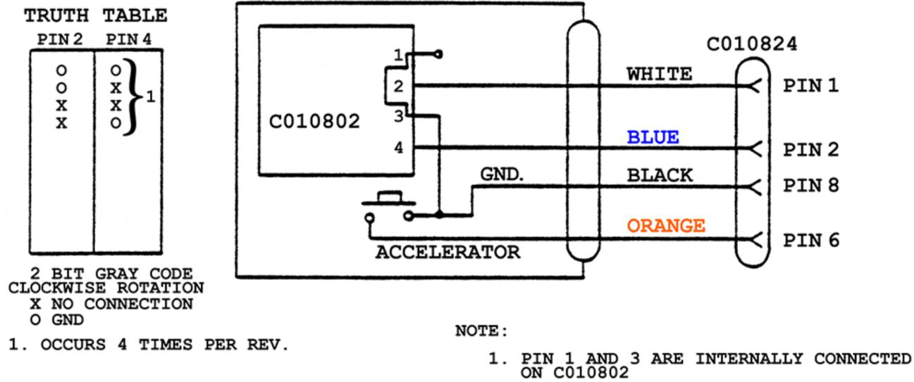
Figure 7-6. Driving Controller Schematic
