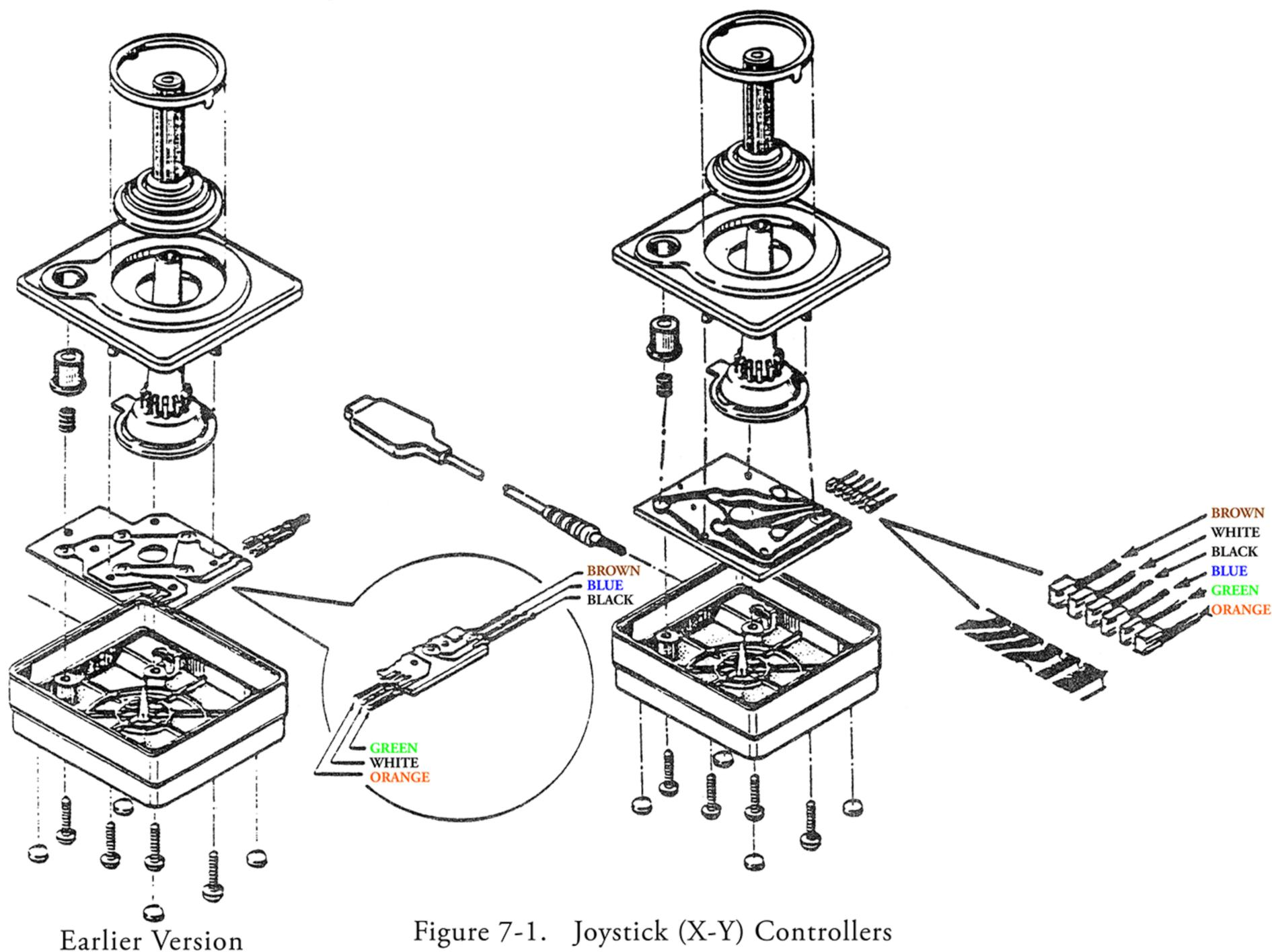
Figure 7-1. Joystick (X-Y) Controllers
