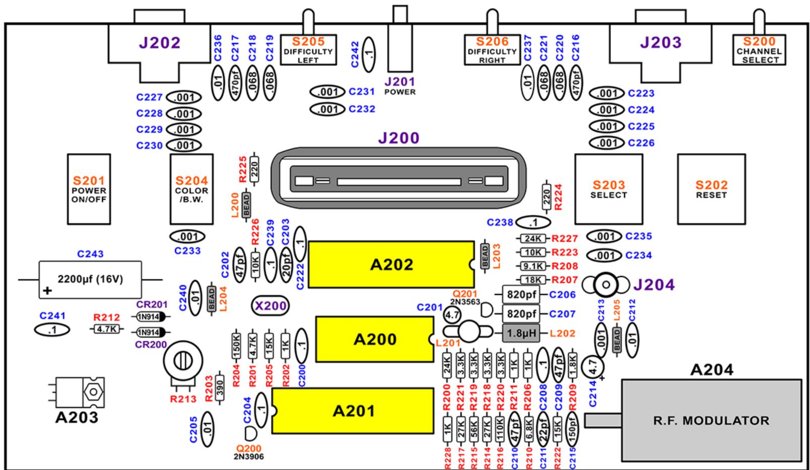
Figure 1-6. 2600A Board Layout (Revs 1-13)
