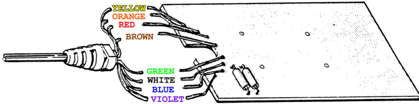
Figure 7-8. Keyboard Wiring Diagram
