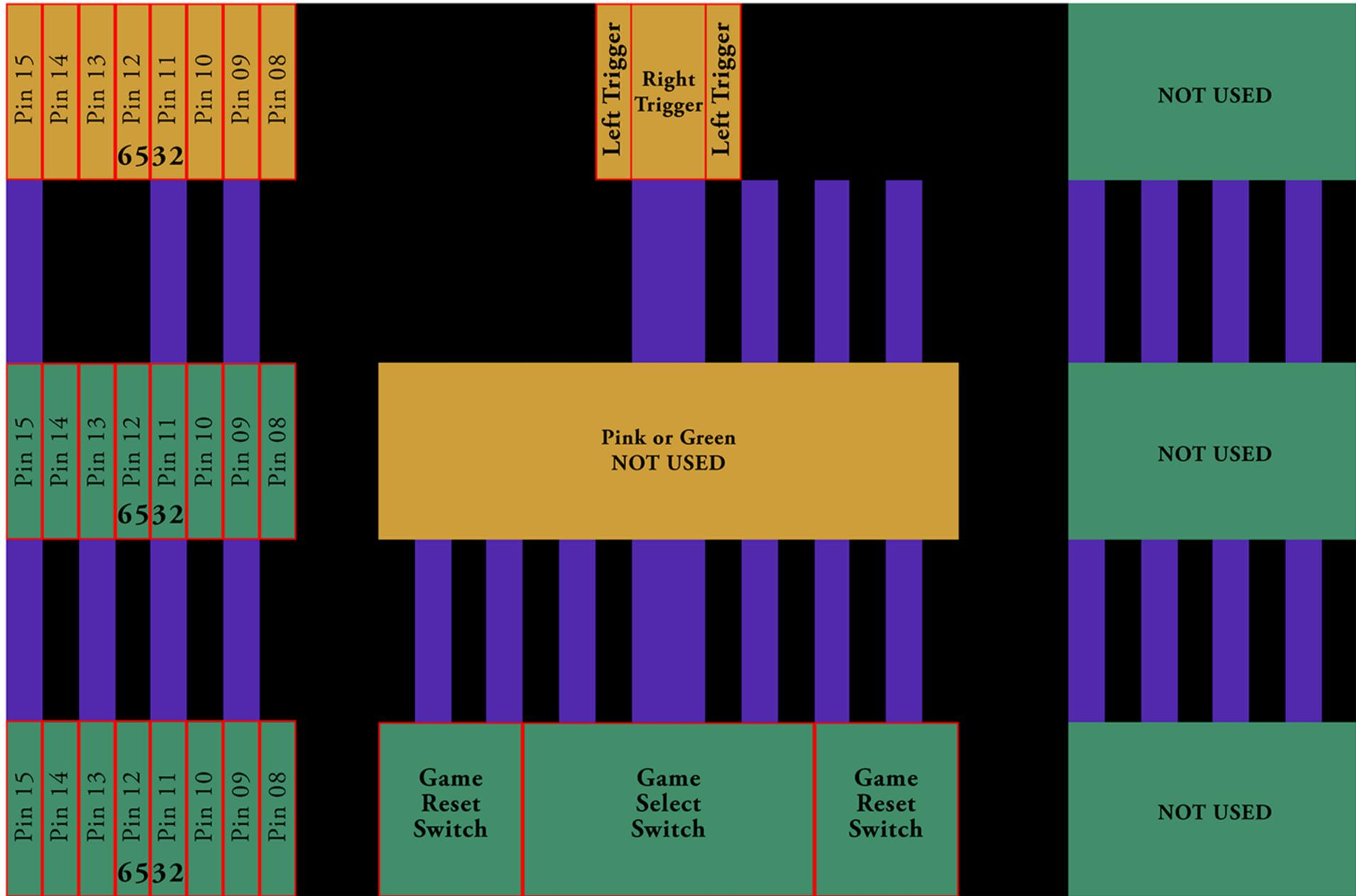
Figure 4-8. Diagnostic Matrix Screen with Defective Pattern
