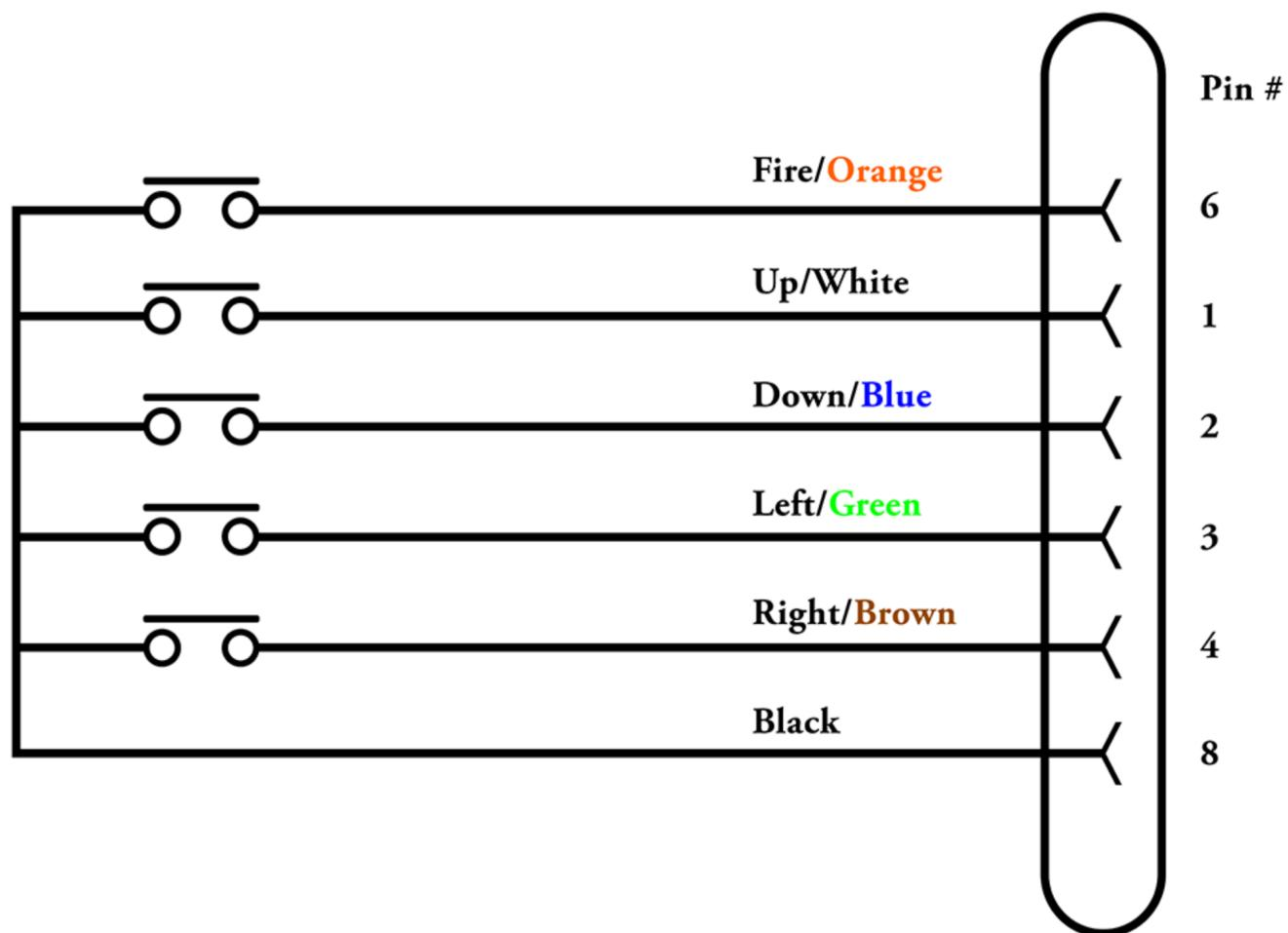
Figure 7-2. Joystick Schematic
