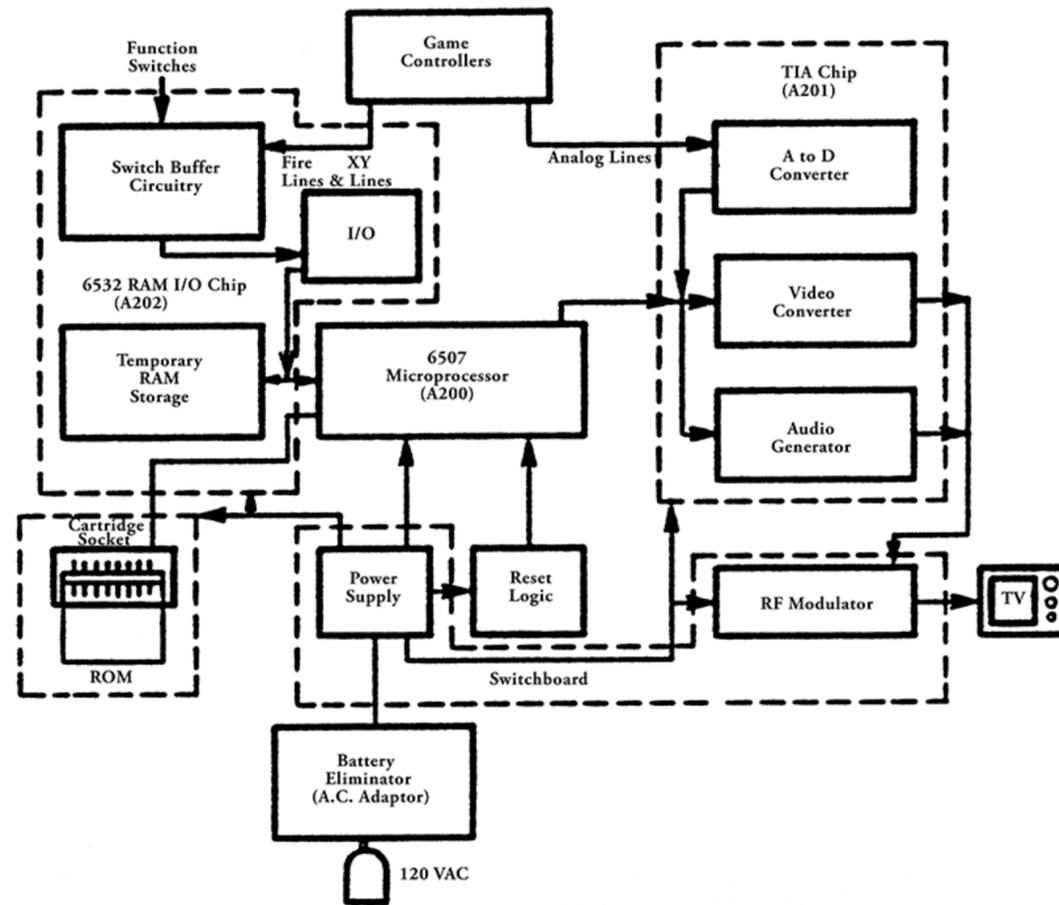
Figure 1-1. 2600 Functional Diagram
