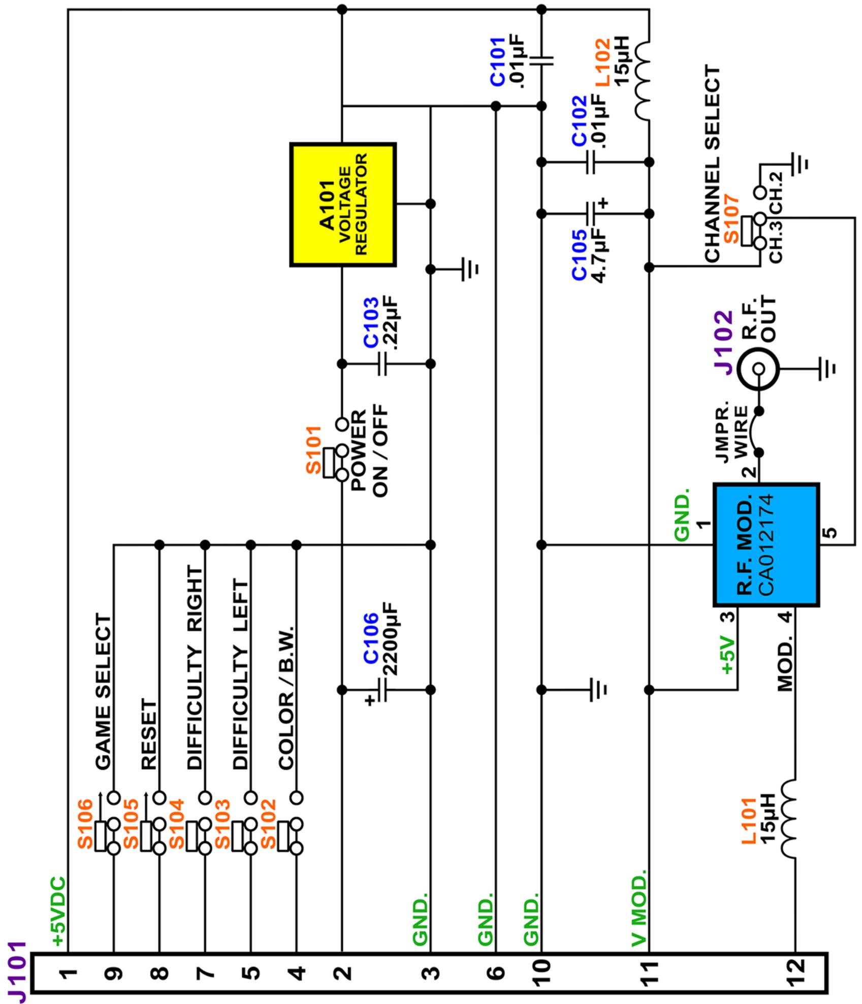
Figure 2-6. 2600 Channel 2-3 Switchboard Schematic
