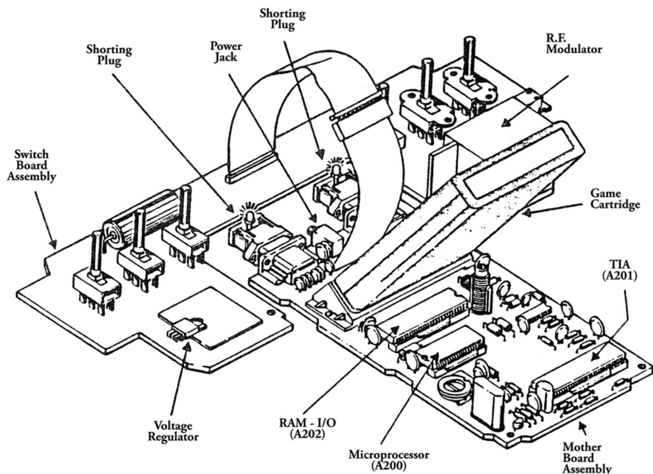
Figure 1-3. 2600 Switchboard and Motherboard Assembly
