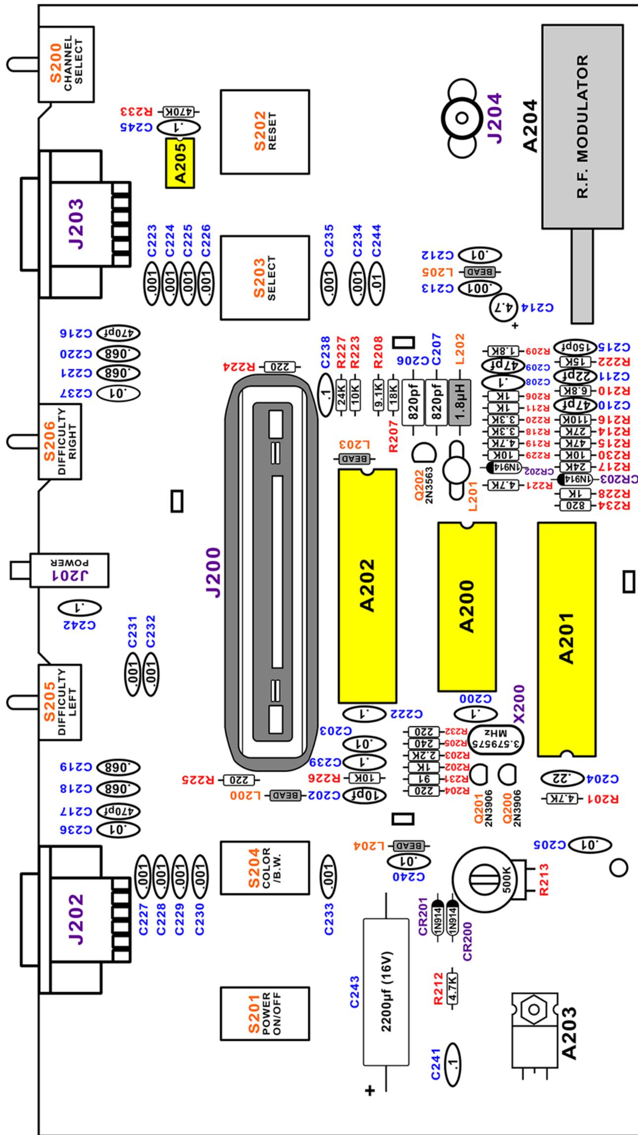
Figure 2-9. 2600A Motherboard Silkscreen (Revs. 16 and up)
