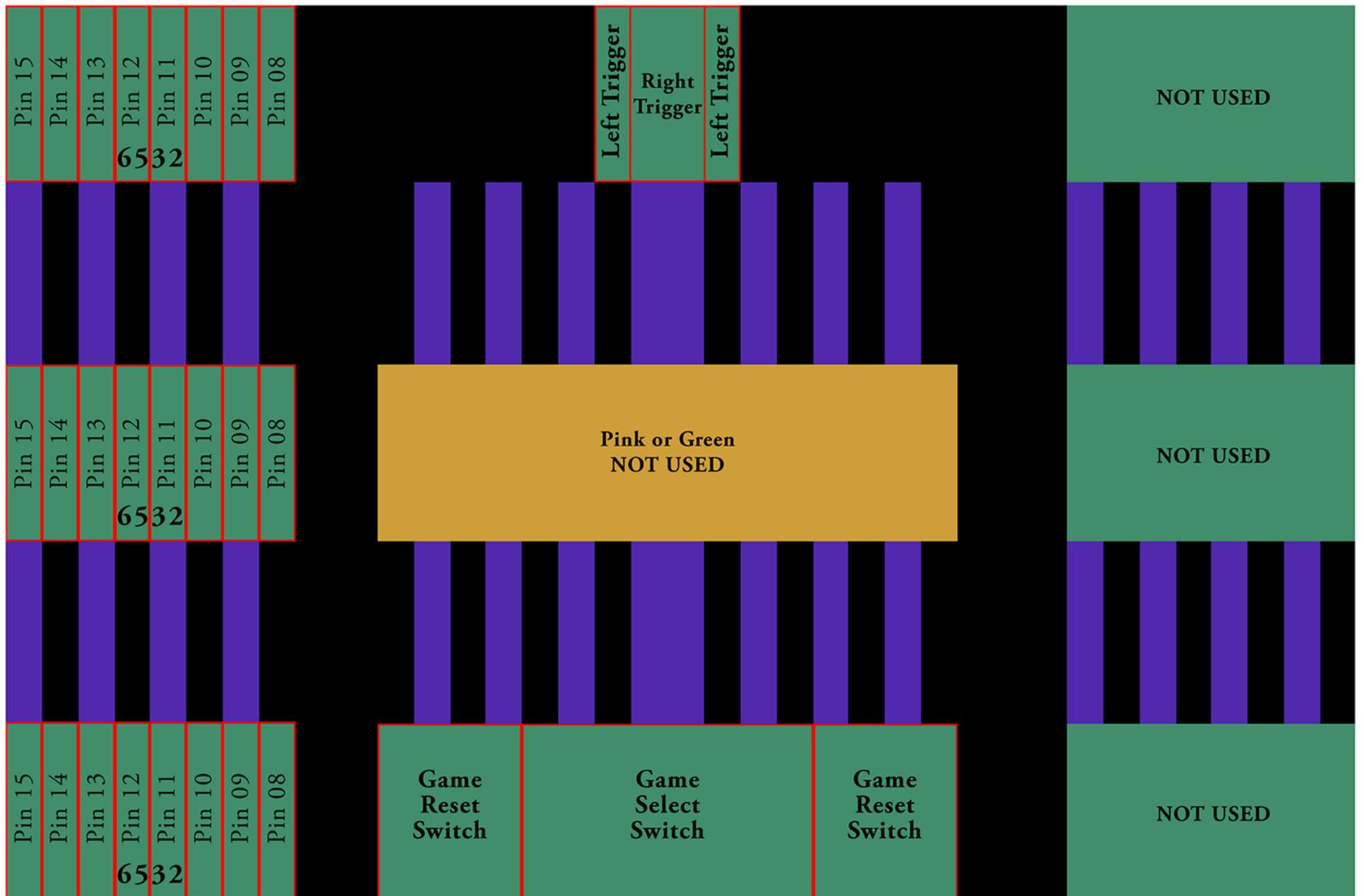
Figure 4-7. Diagnostic Matrix Screen (Shorting Plugs IN)
