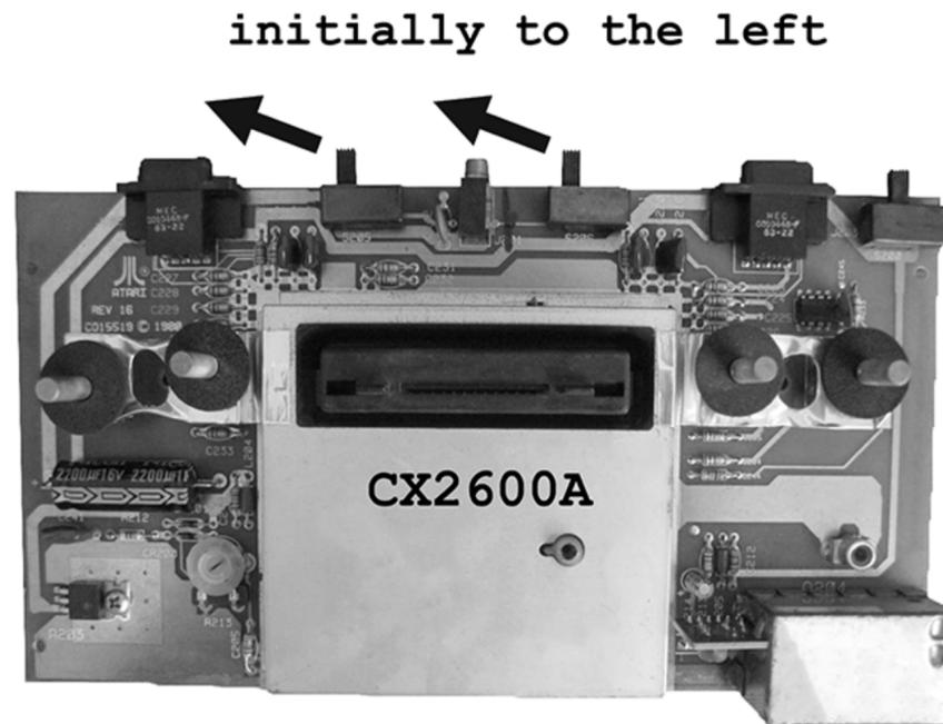
Figure 4-1. Switch Initialization Positions
