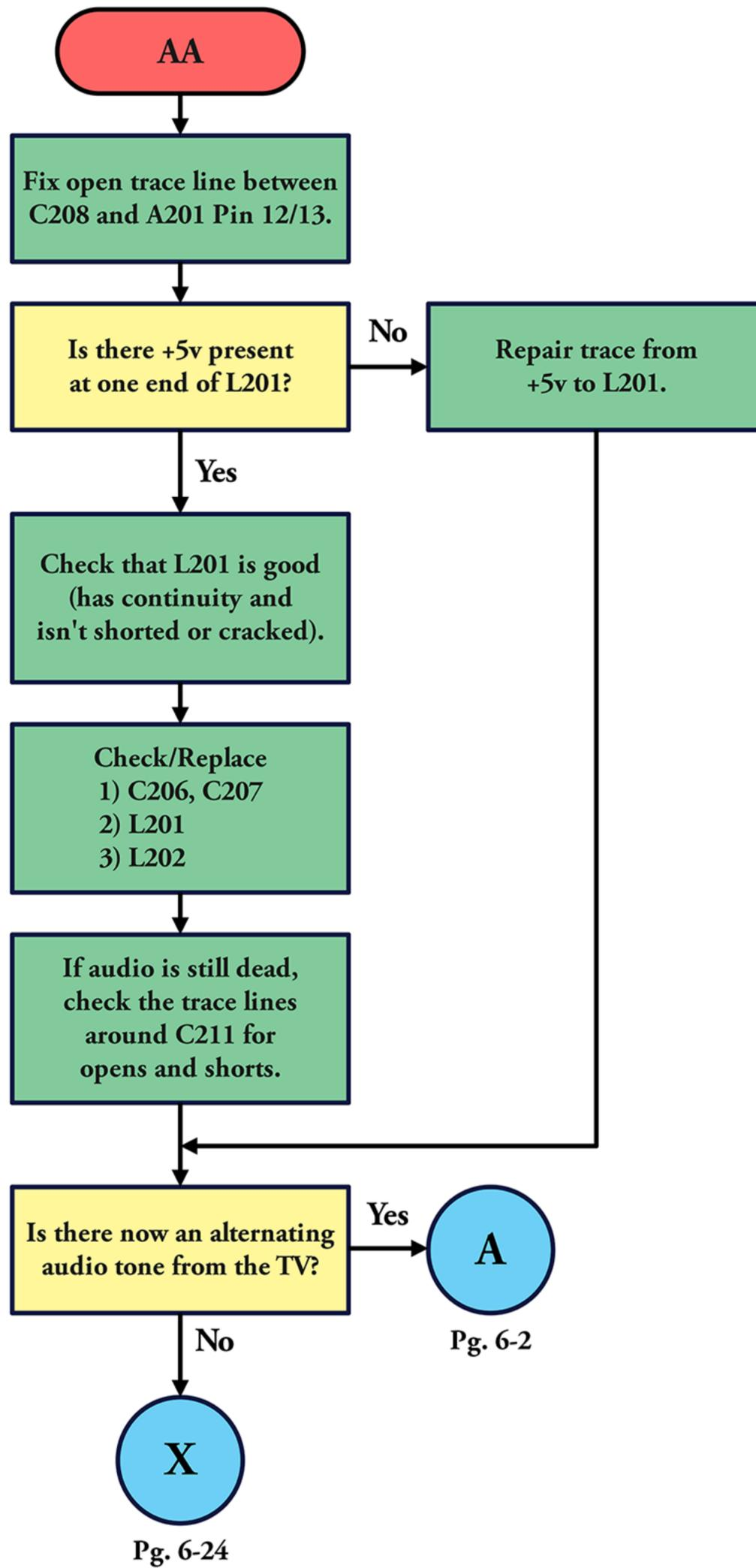
2600A Cartridge Test Procedure
