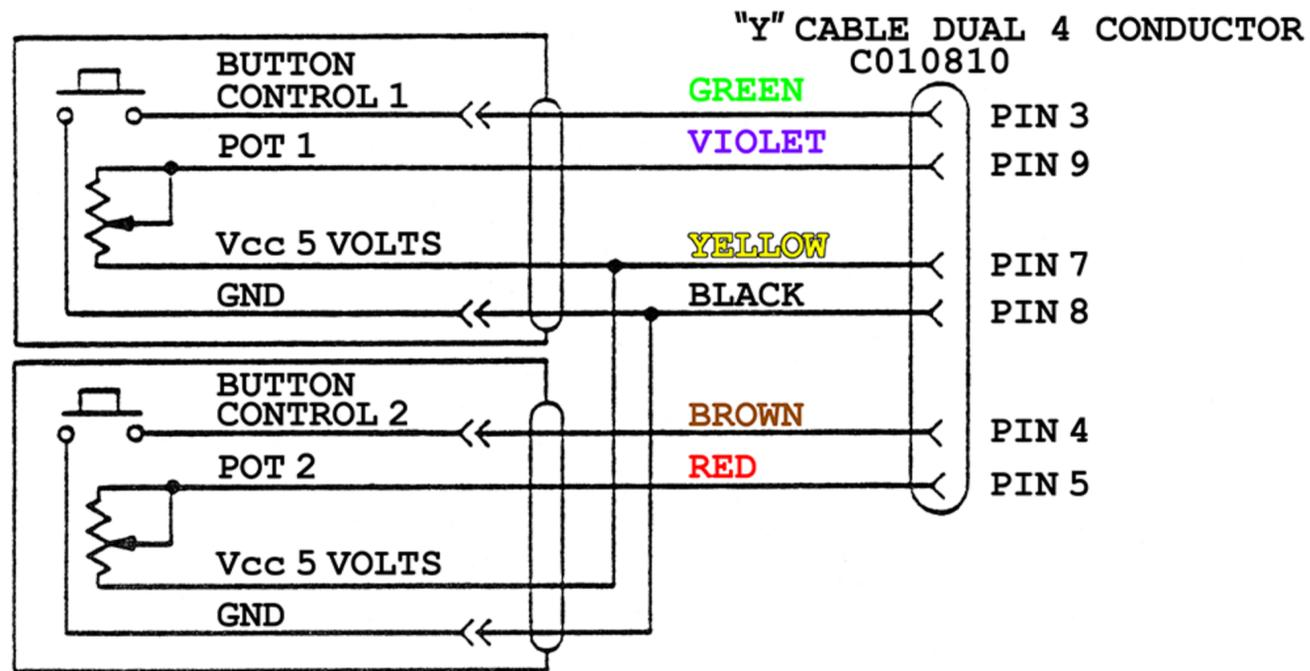
Figure 7-4. Paddle Controller Schematic
